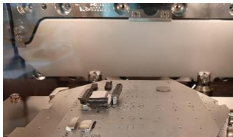
Samples on XPS stage from a mechanical adhesion test.
