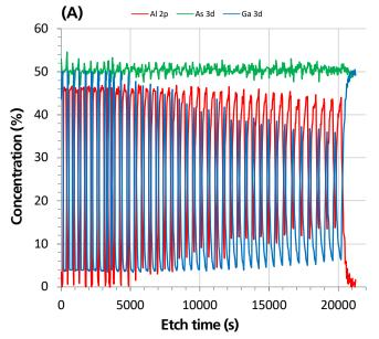
Figure 1A: Complete depth profile of SPLED structure.
