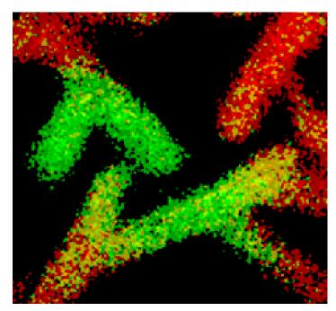
Figure 3: Overlay of C-C and C-OI chemical state images from a PEG-based coating on a PP mesh. Green regions = good coating coverage (C-O), red regions = poor coating coverage (C-C). Image dimensions = 0.8 x 0.8 mm.
