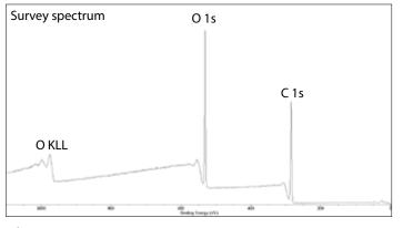
Figure 1: XPS survey spectrum from PEG-coated PP.
