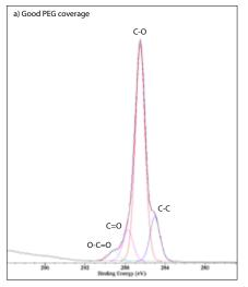
Figure 2a: C 1s XPS spectrum from PP mesh with good PEG coverage.
