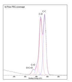
Figure 2b: C 1s XPS spectrum from PP mesh with poor PEG coverage.
